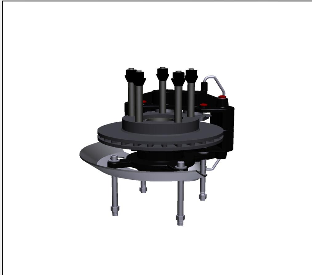
**Warning:** If brake system has been in use, there will likely be some residual brake fluid in the hoses and in the pistons which will leak out with handling. Brake fluid is a category 4 corrosive and will severely damage paint. Brake fluid is also a eye/skin irritant and this procedure should always be done with AEC approved gloves. If fluid is ingested, get to an emergency room immediately.
