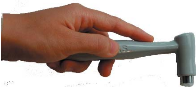
Standard posture of holding the detecting probe. Make sure your hands are dry when you are holding the detecting probe.
