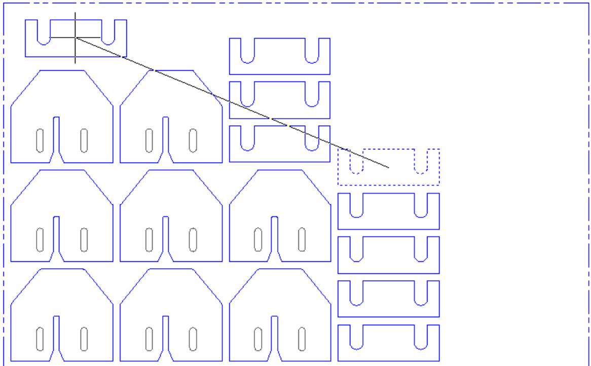
Note. Commands of moving with an index “A” place a part in the way by which allocation of parts has been executed (Rectangle Nesting or Advanced Nesting).
