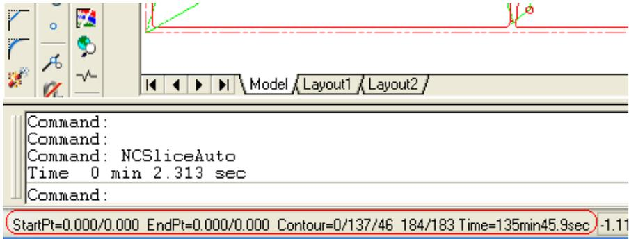
Time=135min 45.9 sec - an estimated cutting time of part contours by the CNC machine tool with current modes cutting.
