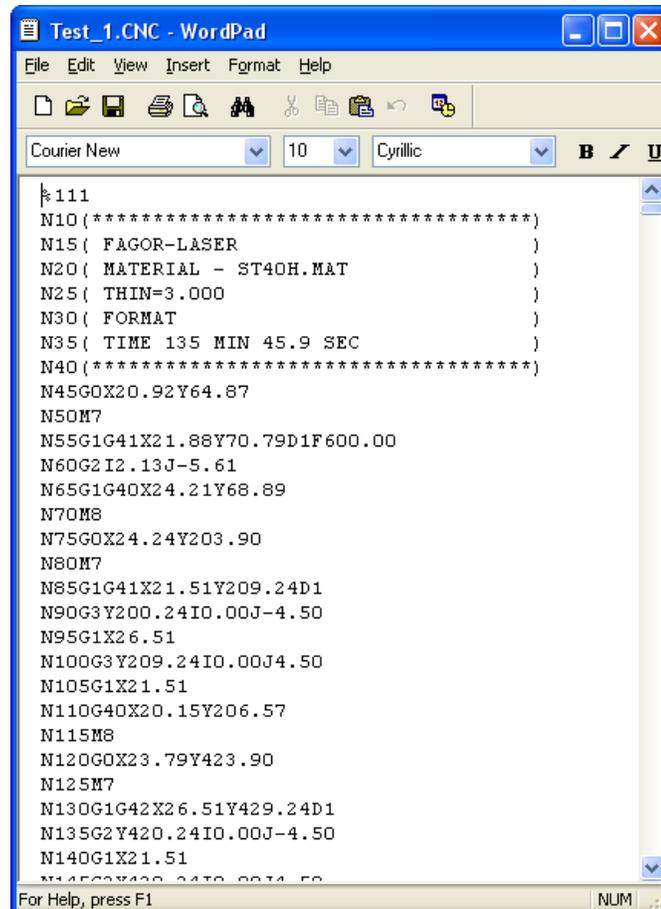
Note. If there is a need to create the program for several machine tools of CNC, execute item 4 selecting a new postprocessor and changing cutting modes.
