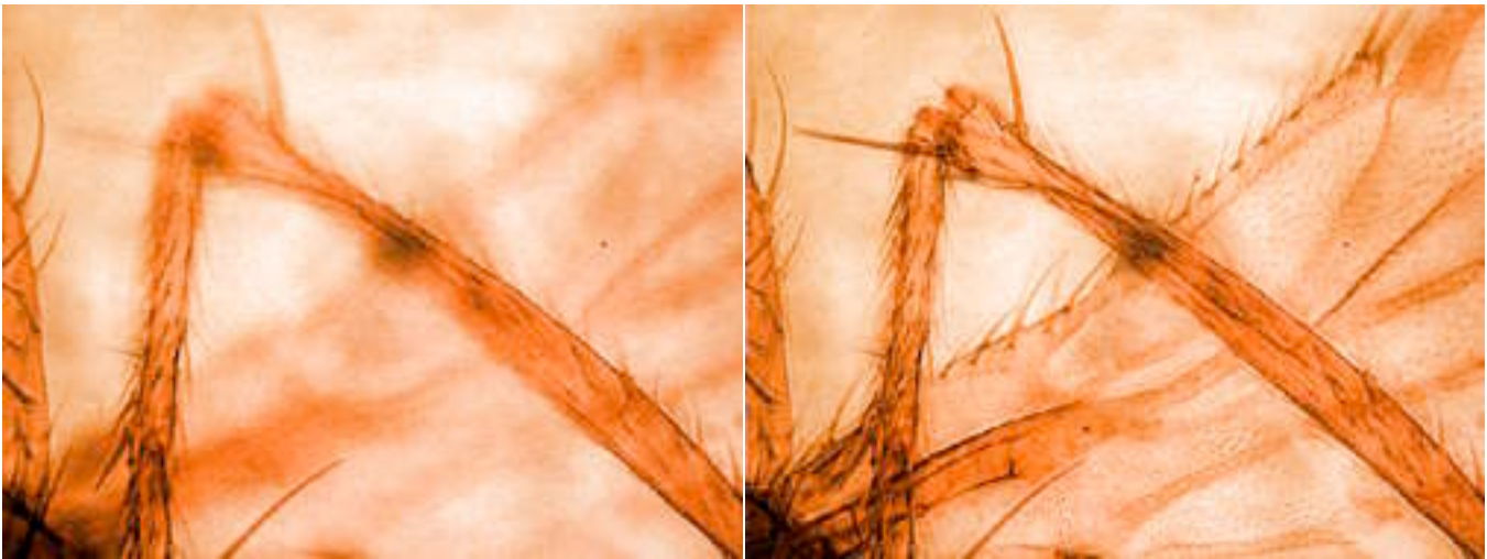
Three light microscope images ( Fly_1,2,3 ) taken by raising the stage to bring different regions into focus, and the composite in which all regions are in focus.
