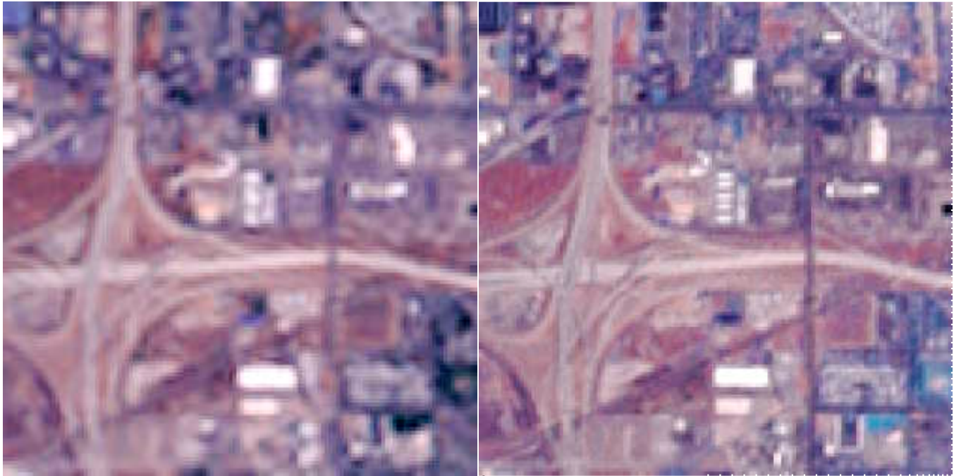
Detail of images formed with RGB channels (left) and inserting high resolution image into I channel (right)
