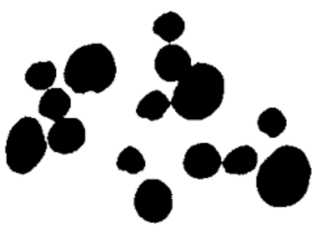
Red channel and thresholded spots with high red intensity
