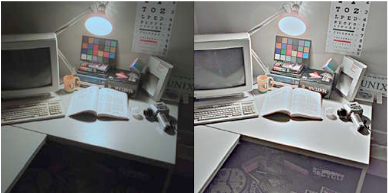
Original Desk image and the result of filtering and histogram shaping.
