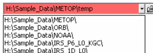
Path to the folder or to the file can be entered manually or via the clipboard by pressing the right mouse button and selecting the corresponding command from the context menu. This context menu also contains commands to copy and delete the text.
