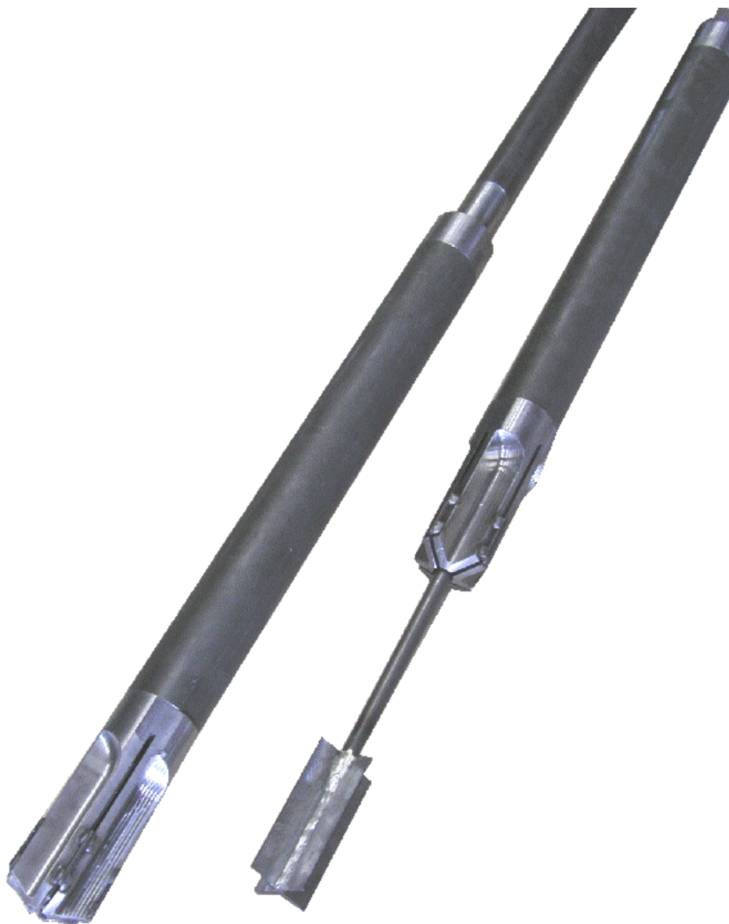
Fig 1.7: Eurocode vane in its protection left and in its extruded position
