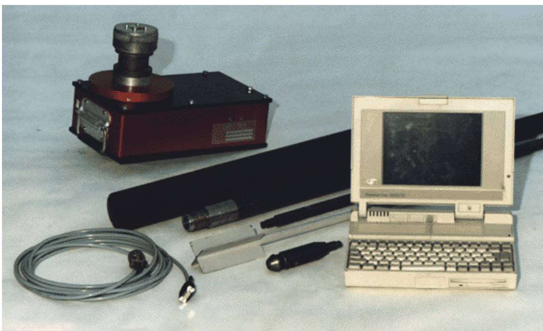
Figure 1.2: Geotech Electrical Vane Test Apparatus, Standard model with (from right to left): Vane with tapered lower end, slip-coupling and extension rod, Instrument Head, IBM compatible PC-computer (not included)
